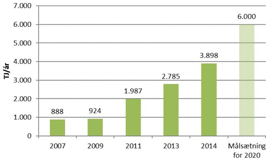
Figure: Onshore wind in Ringkøbing-Skjern Municipality. The figure illustrates the total annual electricity production from onshore wind turbines in Ringkøbing-Skjern Municipality as well as the new target for 2020.
